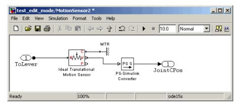
**4** Try to simulate the model. An error message appears saying that the model cannot be compiled because its topology has been changed while in Restricted mode. You can either undo the changes, or switch to Full mode, as described in "Switching from Restricted to Full Mode" on page 4-21.
