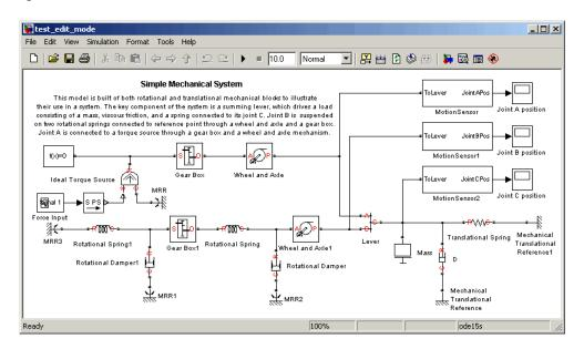
**2** Open the Joint C Position scope and simulate the model. The models runs and simulates in Restricted mode.
