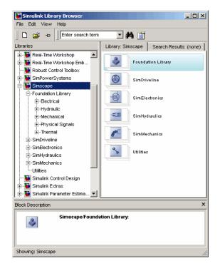
Alternatively, you can type simulink in the MATLAB Command Window. Then expand the **Simscape** entry in the contents tree.
