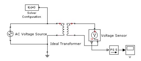
The next diagram would produce an error because it is lacking an electrical reference in the circuit of the secondary winding.
