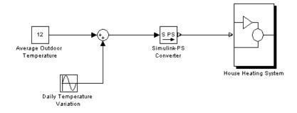
This signal is an absolute temperature reading. Therefore, when the signal converts into kelvin for further computations, you need to specify that it should use affine conversion. Double-click the Simulink-PS Converter block, type C in the **Input signal unit** field, and select the **Apply affine conversion** check box.
