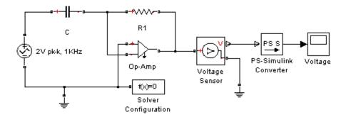
Simulate the model, and you will see that the output is minus the derivative of the input sinusoid.
