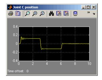
**5** Simulate the model again. Notice that the motion amplitude of node C became smaller as a result of the wheel radius change.
